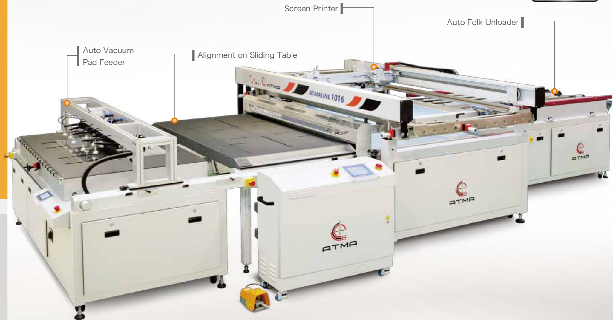
( Automatic feeder – printer – automatic off-loader ) can be collocated freely.
